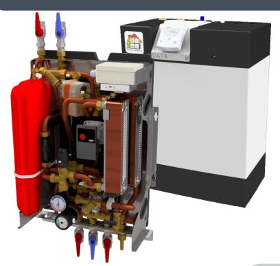
The DATA HIU is suitable for wall hanging in a home or apartment and is designed to provide a range of hot water and central heating outputs using two plate heat exchangers. Within the casing are all controls required for a typical property connected to a district network, including sealed central heating system components with a number of additional options such as hammer arrester, DP valve, and DHW recirculation pump.
